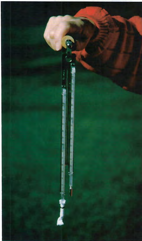
Figure 5 Sling Psychrometer This psychrometer is used to measure both relative humidity and dew point.
