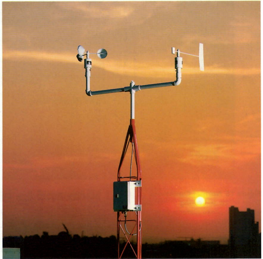
Figure 15 Wind Vane and Cup Anemometer Interpreting Photographs How does the position of a wind vane tell you which direction the wind is blowing?
