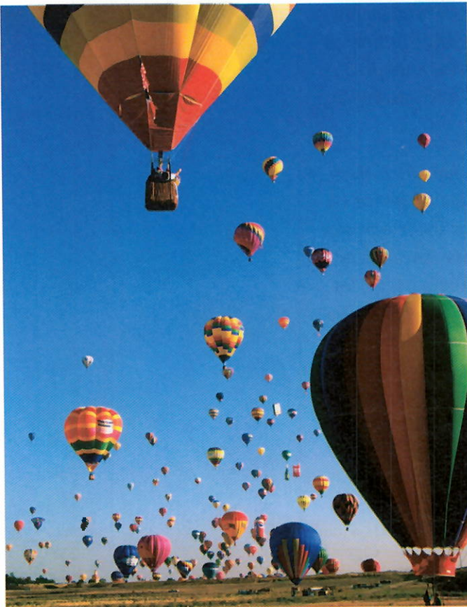
Figure 9 Hot-air balloons will rise as long as the air inside them is warmer than the air in the atmosphere surrounding them.
