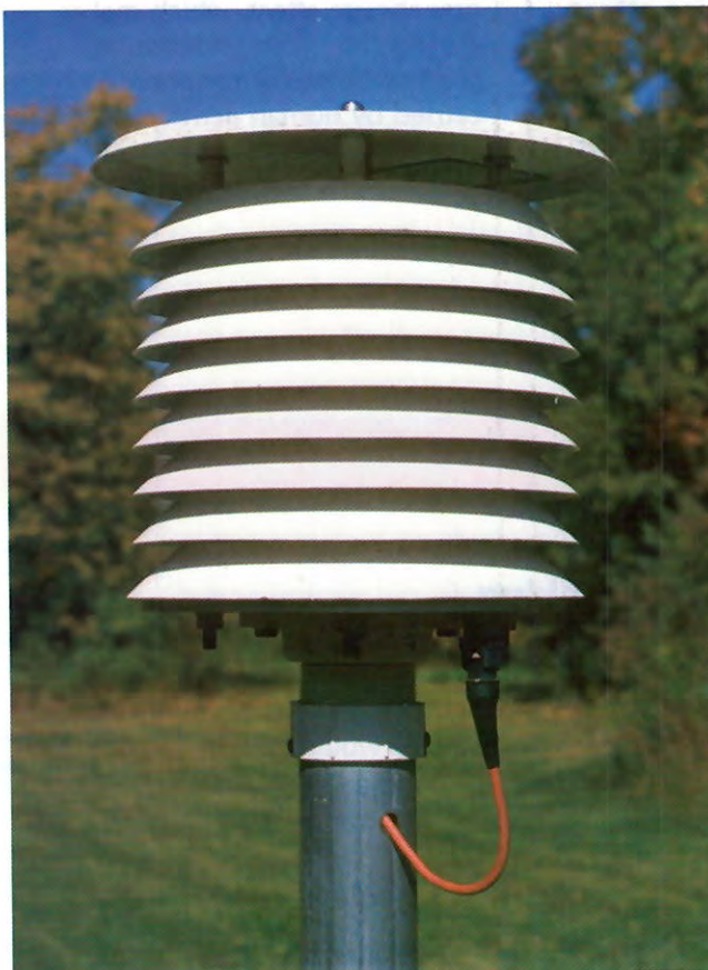
Figure 14 This modern instrument shelter contains an electrical thermometer called a thermistor.
