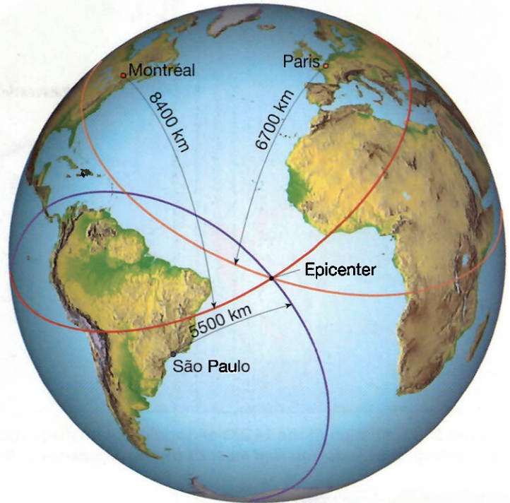
Figure 8 Locating an Earthquake A A travel-time graph is used to determine the distance to the epicenter. The difference in arrival times of the first P wave and the first S wave in the graph is 5 minutes. So the epicenter is roughly 3800 kilometers away. B The epicenter is located using the distance obtained from three seismic stations. The place the circles intersect is the epicenter.
